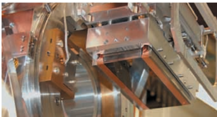
Optics for Tomography Beamline at Swiss Light Source
