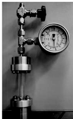
Figure 1: Sapphire single crystal gas pressure cell under hydrogen pressure
