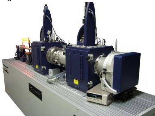
Rigaku S-MAX 3000™ with dual sample chamber and offset detector position
